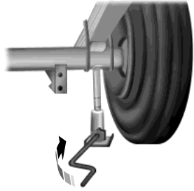
Rear axle jacking points - All models except E-350 dual rear wheel and E-450
